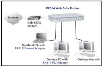
This image shows the flow of data to multiple computers sharing one high speed Internet connection.
