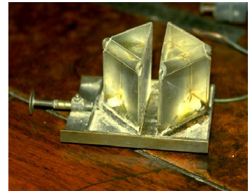
Figure 14. One of Bose's original double-prism attenuators, with adjustable air gap.
