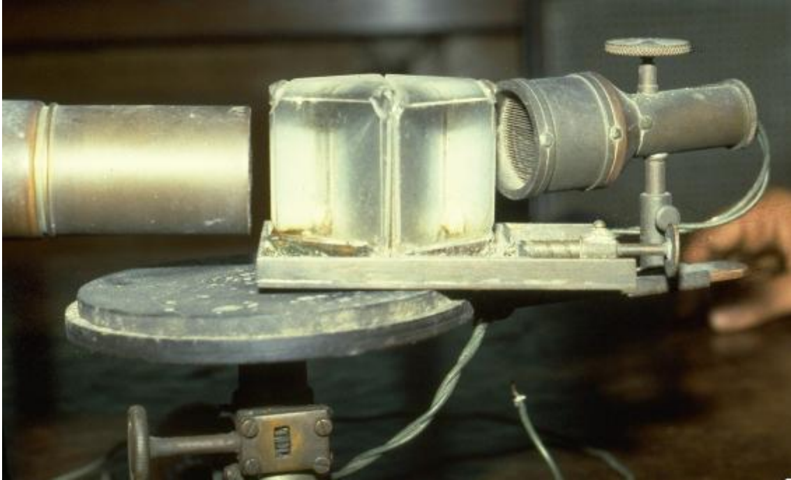
Figure 4(c) A complete setup showing the transmitting antenna at the left, with the receiving antenna at right. Note the adjustment screw on top of the receiving antenna, which is used to adjust the pressure of the point-contact detector (see Fig. 5). In the center is a rotating table (the "spectrometer circle" of Figure 2) on which various microwave components (prisms, lenses, grids, polarizers etc.) may be mounted for study. A dual-prism attenuator (see below) is shown in this photograph. The arrangement as shown is not yet properly aligned.
