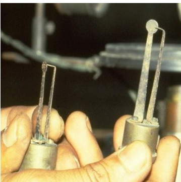
Figure 5. Two of Bose's point contact detectors, removed from the receiving antennas.
