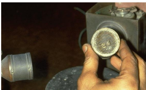
Figure 4(a) One of Bose's transmitter antennas (being held on the right of the picture). Note the polarizing grid; the spark gap is just visible behind the grid. In the background behind this antenna part of the high voltage equipment used to generate the spark can be seen. At the left of the picture is a receiving horn.
