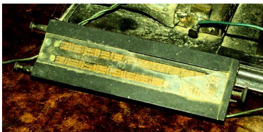
Figure 8. One of Bose's free-space radiation receivers, recently described as a "space-irradiated multi-contact semiconductor (using the natural oxide of the springs)." The springs are kept in place in their tray by a sheet of glass, seen to be partly broken in this photograph.
