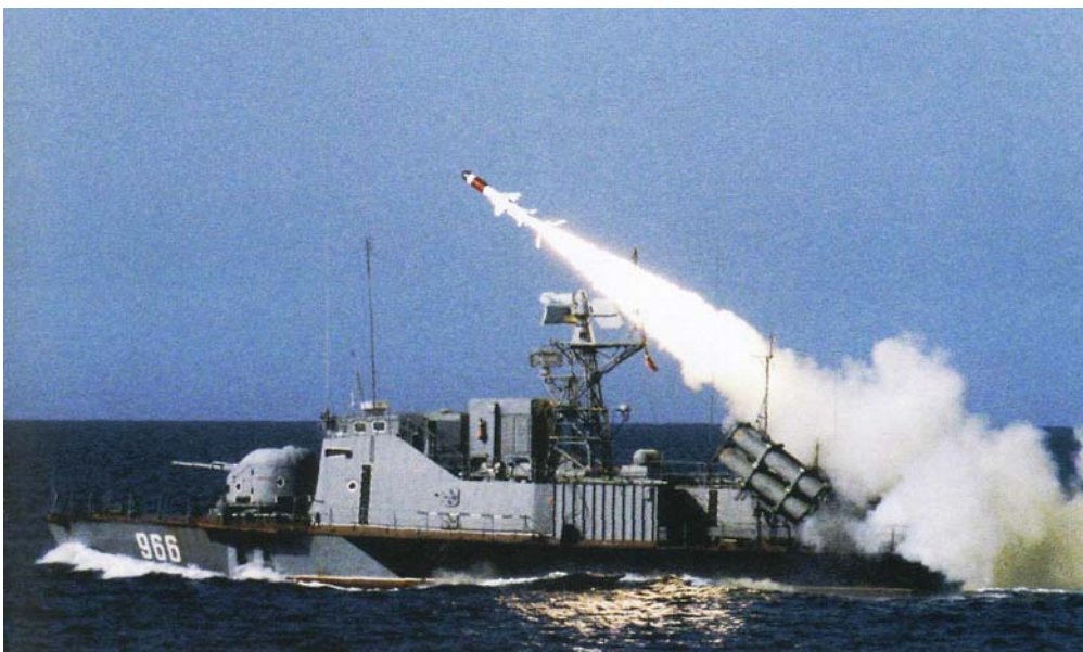
Start of the anti-ship missile X-35E with a radar seeker ARGS-35E made by JSC "Radar MMS", 2002
