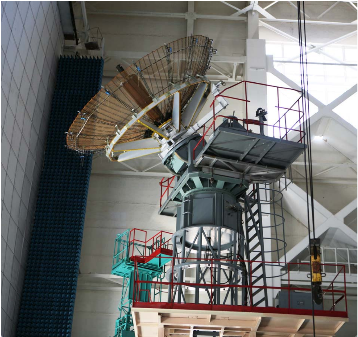
Satellite antenna on the test bench
