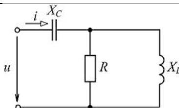
$$\dot{Z}_{\text{вх}} = 10 + j10 \text{ Ом}, \varphi = 45^\circ.$$
