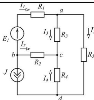
$$I_1 = -1 \text{ А}, I_5 = 2 \text{ А}, I_4 = 6 \text{ А}.$$
