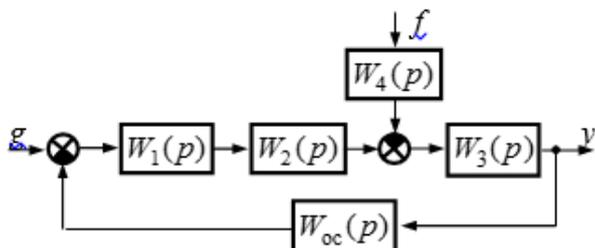
$$W_1(p) = \frac{k_1}{T_1 p + 1}, \quad W_2(p) = \frac{k_2}{T_2 p + 1},$$
