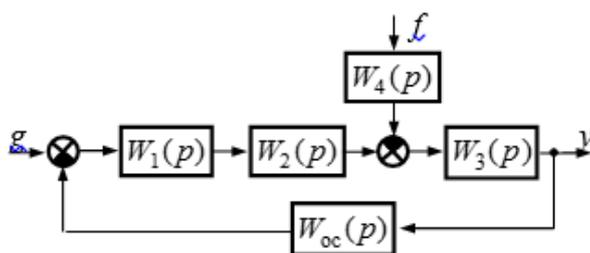
$$W_1(p) = \frac{k_1}{T_1 p + 1}, \quad W_2(p) = \frac{k_2}{T_2 p + 1},$$
