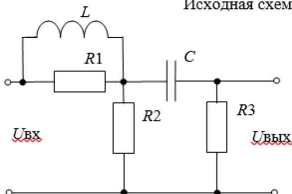
$$\begin{aligned} R1 &= 100 \text{ Ом} \\ R2 = R3 &= 10 \text{ кОм} \\ C &= 0,5 \text{ мкФ} \\ L &= 0,6 \text{ Гн} \end{aligned}$$
