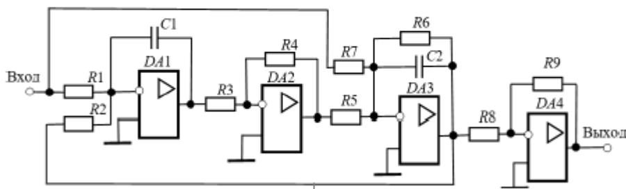
$$R_1 = R_2 = 1,25 \text{ МОм}, \quad R_3 = 200 \text{ кОм}, \quad R_4 = R_5 = 10 \text{ кОм}, \quad R_6 = 625 \text{ кОм}, \quad R_7 = 1,25 \text{ МОм},$$
