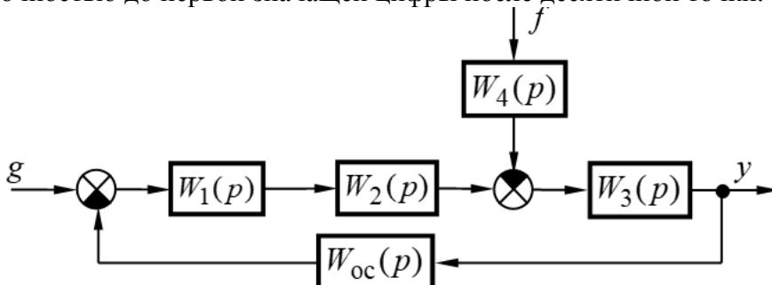
$$W_1(p) = \frac{k_1}{T_1 p + 1}, \quad W_2(p) = \frac{k_2}{T_2 p + 1}, \quad W_3(p) = \frac{k_3}{T_3 p + 1}, \quad W_4(p) = k_4, \quad W_{\text{oc}}(p) = \frac{k_{\text{oc}} p}{T_{\text{oc}} p + 1};$$
