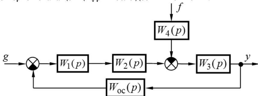
$$W_1(p) = k_1, \quad W_2(p) = \frac{k_2(\tau_2 p + 1)}{T_2 p + 1}, \quad W_3(p) = \frac{k_3}{T_3^2 p^2 + 2\xi T_3 p + 1}, \quad W_4(p) = k_4,$$
