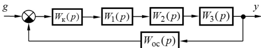
$$W_1(p) = \frac{k_1}{T_1 p + 1}, \quad W_2(p) = \frac{k_2}{T_2 p + 1}, \quad W_3(p) = k_3, \quad W_{\text{oc}}(p) = k_{\text{oc}},$$
